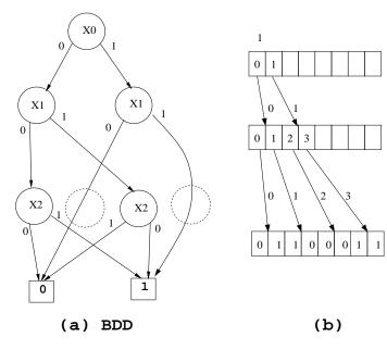
**Figure 1.** (a) BDD for the Boolean logic function  $f = x_0 \cdot x_1 + \bar{x_0} \cdot (\bar{x_1} \cdot x_2 + x_1 \cdot \bar{x_2})$ . (b) Representation of the BDD in memory.
